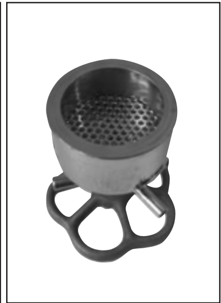
Figure 4. BHS Pocket-Leaf Filter for bench-top testing for filtration, washing and drying studies.
