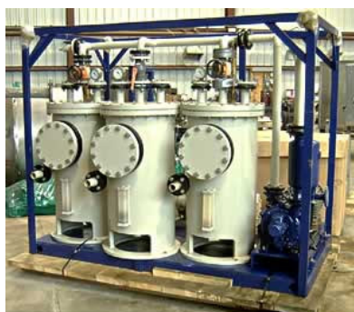
Vacuum and Filtrate Skid
