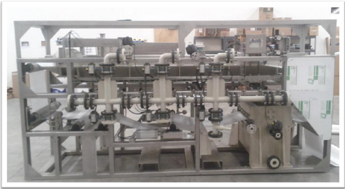
Figure 6: BHS Vacuum-Filtrate Skid for BF 025-024 (0.6 m2 filter area)
