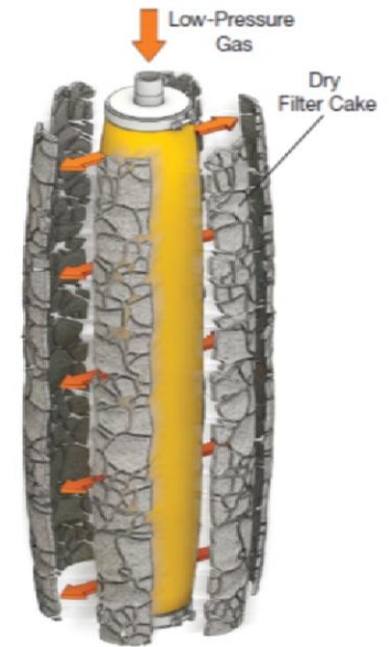
▲ Figure 3. During discharge, gas is fed into the top of the candle, which expands the flexible filter sock. This causes the dry cake to crack and break away from the filter. The solids are collected at the bottom of the pressure vessel.
