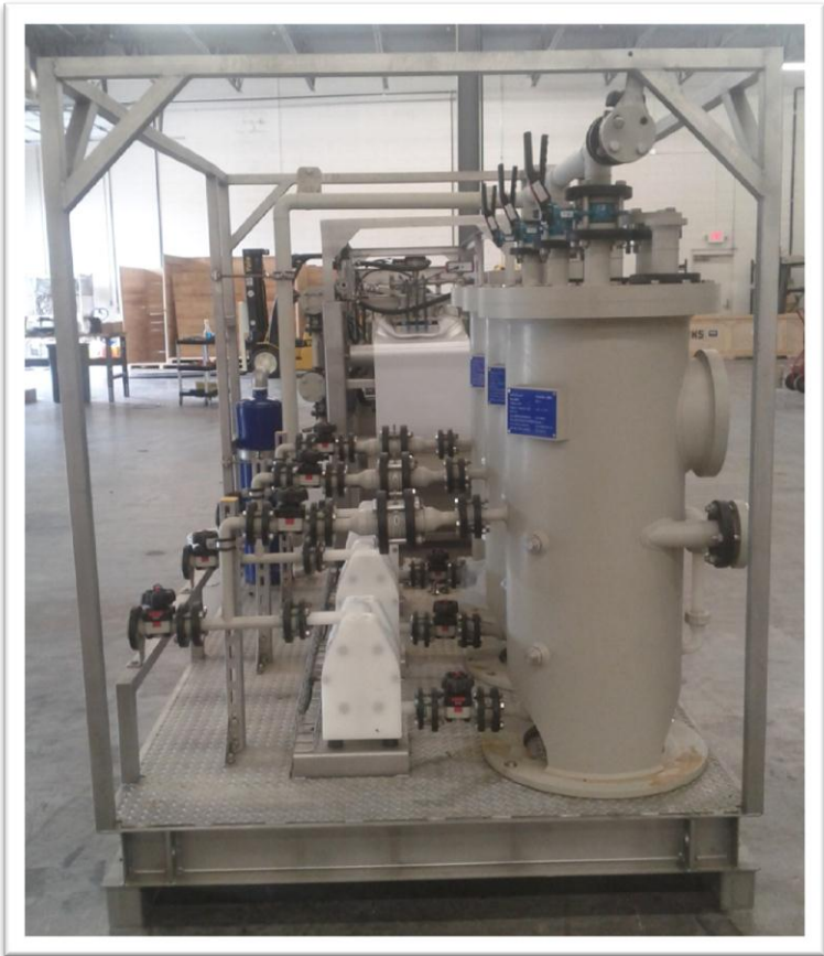
Figure 6: BHS Vacuum-Filtrate Skid for BF 025-024 (0.6 m2 filter area)
