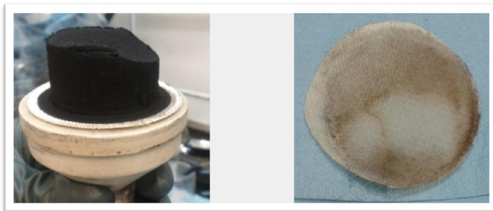
Figure 4: Cake Structure and Cake Discharge from Vacuum Filtration
