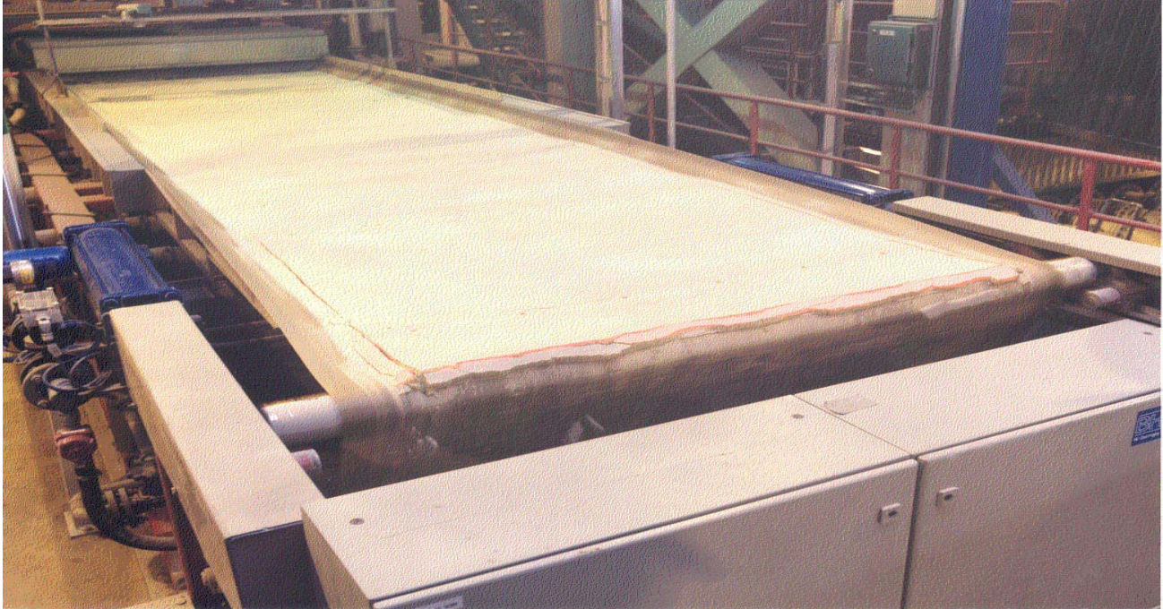
Figure 3: Continuous-Indexing Belt Filter with 12 m 2 of Filter Area Installed for a Gypsum Dewatering System Producing 9000 Kilograms/Hour of Dry Gypsum
